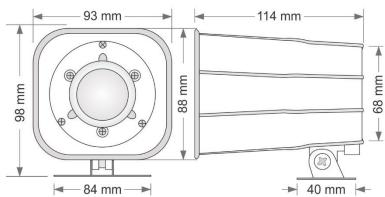
All dimension are in mm tolerance ±0.2mm
