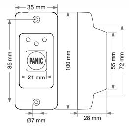
All dimension are in mm tolerance ±0.2mm
