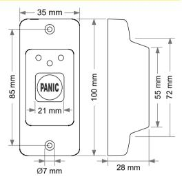
All dimension are in mm tolerance ±0.2mm
