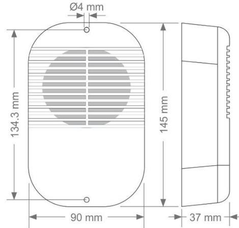
All dimension are in mm tolerance  $\pm 0.2\text{mm}$
