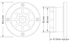
All dimension are in mm tolerance ±0.2mm
