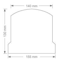
All dimension are in mm tolerance ±0.2mm
